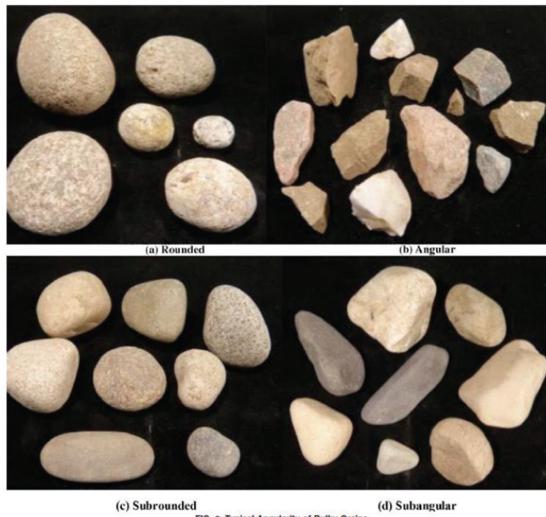
FIG. 3 Typical Angularity of Bulky Grains
